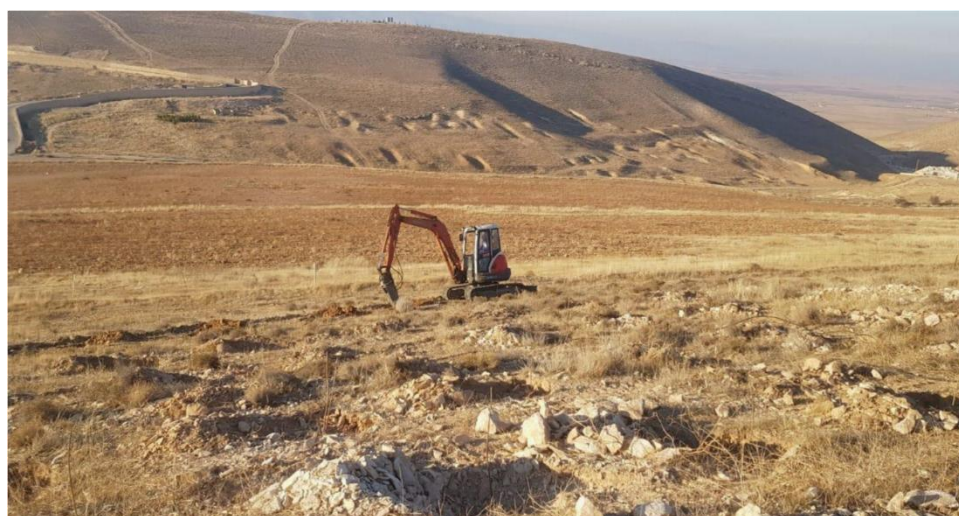
Fig 4.11: Excavating holes with a small backhoe at Ras Baalbek for fall planting
